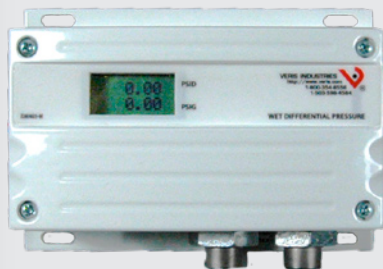
3-wire pressure transducer, field-selectable output — 0-5V/0-10VDC or 4-20mA. LCD displays gauge and differential pressure
