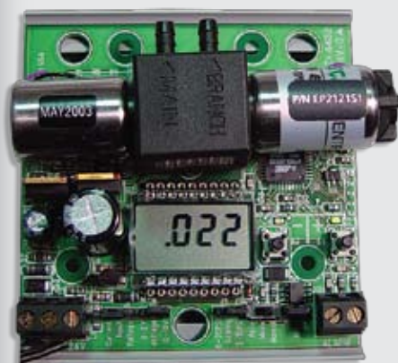
Equipped with jumper selectable control ranges (0-20 psig or 3-15 psig)
