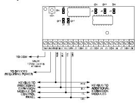
**TAM** - This can be used to tamper the cabinet that the PC5108FLR is mounted in. Connect a normally closed (NC) switch across TAM and BLK. If the tamper is not being used, connect a piece of wire across TAM and BLK to remove the trouble condition.
