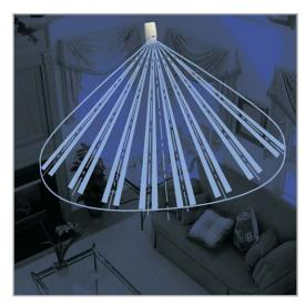
The anti-masking feature prevents intruders from defeating the detector by covering its field of view.
