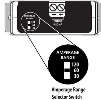
2. Scale controller software to match selected output.
