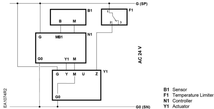
**Figure 19. Terminal Connections.**
