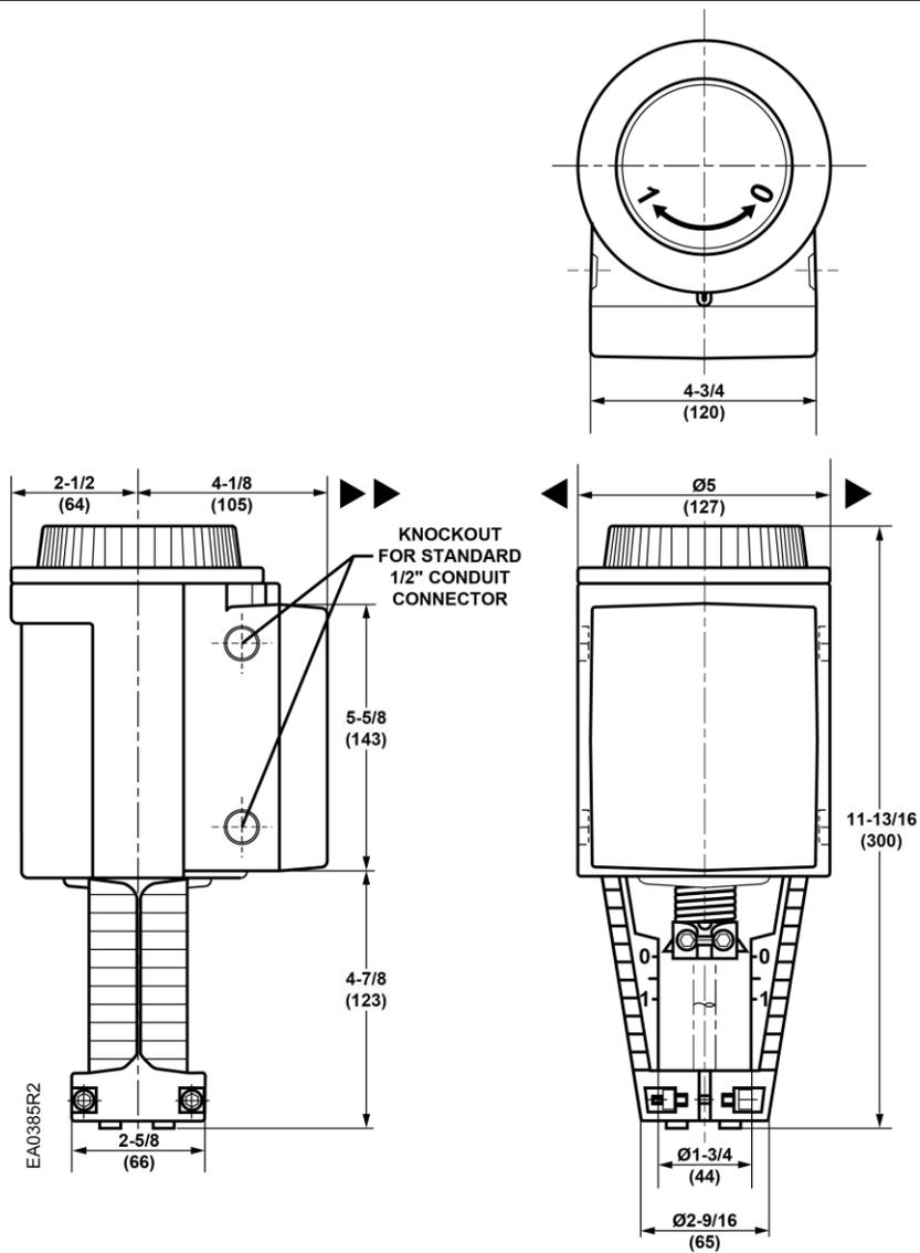
**Figure 26. Dimensions of SKD Actuator in Inches (Millimeters).**
