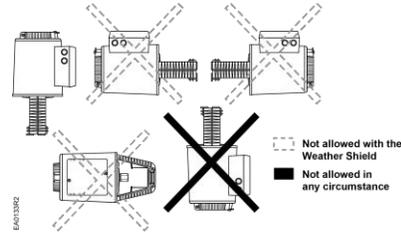
**Figure 10. Acceptable Mounting Positions.**
