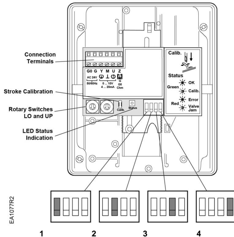
Figure 13. DIP Switches.
