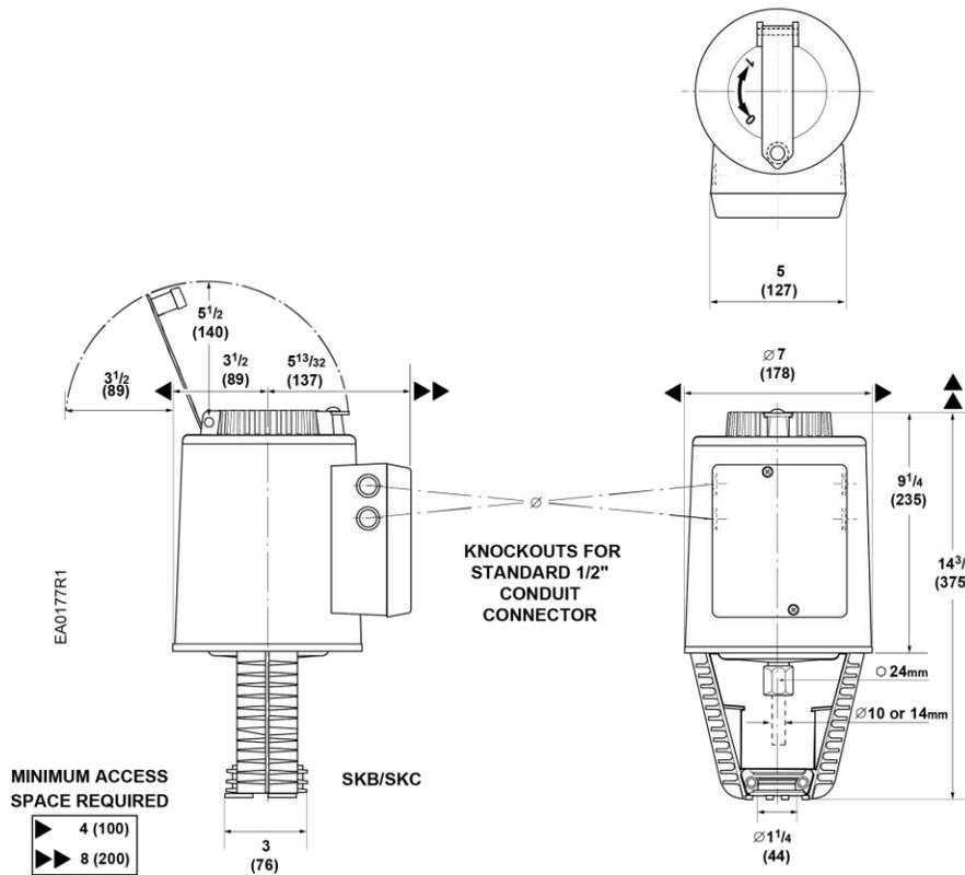
**Figure 25. Dimensions of SKB/C Weather Shield, 599-10071 in Inches (Millimeters).**
