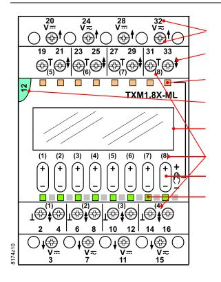
Connection terminals (No. 1 screwdriver for slotted or recessedhead \* screws) with test pickup (for 1.8...2 mm pins) and terminal number Signal designation
