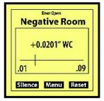
If pressure is Normal, and Door is open, the screen is Yellow
