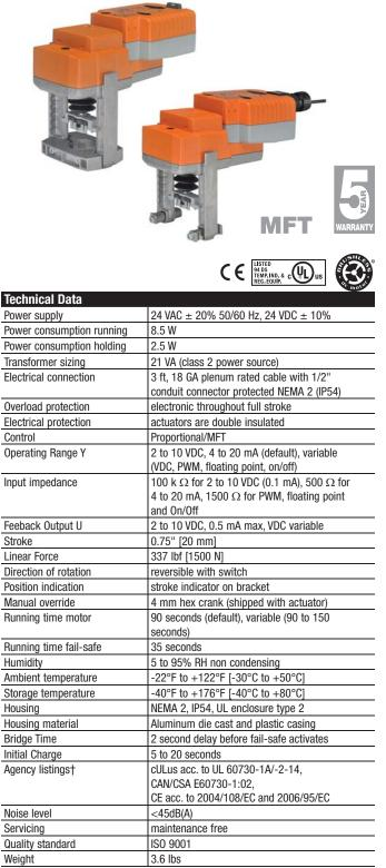
† Use flexible metal conduit. Push the Listed conduit fitting device over the actuator's cable to butt against the enclosure. Screw in conduit connector. Jacket the actuators input wiring with Listed flexible conduit. Properly terminate the conduit in a suitable junction box. Rated impulse Voltage 800V. Type of action 1. Control Pollution Degree 3.
