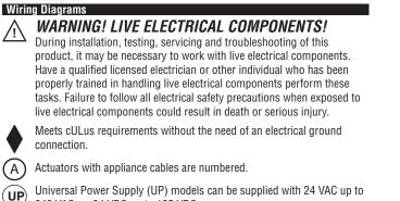
Universal Power Supply (UP) models can be supplied with 24 VAC up to 240 VAC, or 24 VDC up to 125 VDC.
