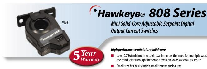
The **Hawkeye 808 Series** is a high performance miniature solid-core current status switch. Its low minimum setpoint (0.75A) and small size make it ideal for monitoring status of small to medium motor loads. With an amperage range of 0.75 to 50 amps, the 808 series can accurately detect belt loss, coupling shear, or other mechanical failure on loads from 1/5 to 40HP.
