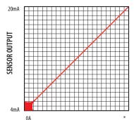
SENSED AMPS \*Adjusted with Span Potentiometer for Hx21 models; Factory-set per customer specification for Hx21SP models
