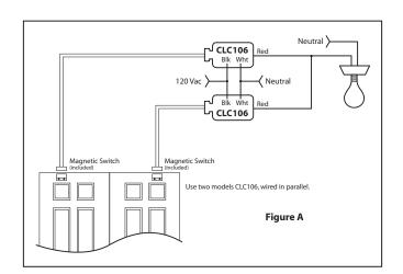
Always follow NEC® and local codes. Functional Devices, Inc. recommends adding a label on each device used in this application with the message: "WARNING – LOAD SIDE TERMINALS MAY BE ENERGIZED BY BACKFEED," similar to what is recommended in NEC® Article 404.6 (C) 2008.
