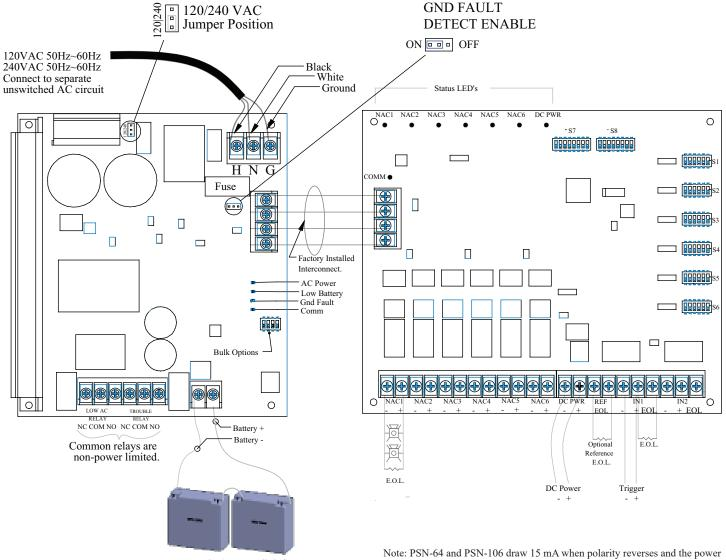
Battery connection (non-power limited). Use two (2) 12V batteries connected in series.
