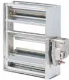
Smoke dampers do not always require a sleeve for proper installation. External installation of the actuator can be provided using a sideplate (usually the full height of the damper). These dampers are installed in a slotted duct section with the sideplate covering the slot in the side of the duct. However, full-height sideplates may not be practical on large smoke damper (particularly multi-section assemblies).
