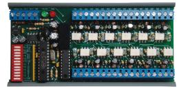
TWO (ACCUMULATOR) INPUTS CAN BE USED FOR POWER MONITORING OR OTHER PULSE COUNTING APPLICATION.
