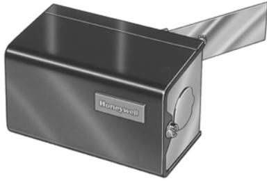
The S437 and S637 Sail Switches respond to the air velocity in heating or warm air ducts, such as used in farm crop dryers. The switch completes a 24V or line voltage burner control circuit only when the blower or fan has produced a predetermined air velocity.
