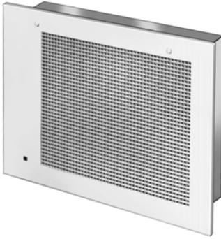
The F52F Return Grille Electronic Air Cleaner is wall or ceiling mounted in the main return air duct of a central forced air heating, cooling, or ventilation system. It captures a significant number of the airborne particles (0.5 microns and larger) from the air circulated through the cell(s).
