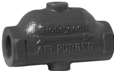
Air Purgers provide efficient separation of air and water in hydronic heating systems. Heavy duty cast bronze construction with tappings for expansion tank and automatic air vent mountings. Removes entrapped air with internal baffle design through continuous recirculation of heating system water with use of air vent. Improves system efficiency, reduces noise and helps extend component life.
