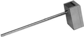
**The H7015B Combined Humidity/Temperature Duct Sensor combines a capacitance-type relative humidity sensor with a PT1000 or BALCO 500 temperature sensor in one housing. These sensors can be used for discharge, outside or return air control or as a high-limit sensor in applications such as steam humidification.**
