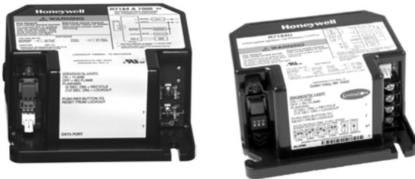
Line voltage, safety rated, control for residential oil fired burners used in boilers, forced air furnaces and water heaters. When used with a cad cell flame sensor, operates an oil burner and optional oil valve. Can be used with both hydronic and forced air systems.
