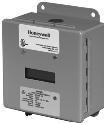
The Class 500 Meter is a 3-element meter with communications. The device is used to monitor electric power usage of individual loads after the utility meter and store kW and kVAR data for automatic meter reading. Installation must only be performed by qualified personnel and in accordance with these instructions and all applicable local and national electrical codes.
