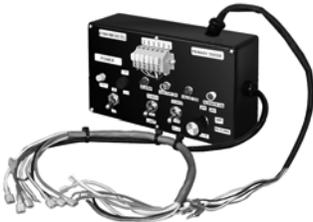
The A7184 Cad Cell Primary Tester is a convenient on-the-job tester that can be used for all R8184 and R7184 Cad Cell Primaries. It lets the service technician check out the primary quickly and easily by simply connecting it to the tester and plugging the tester into a standard 120 or 240 volt ac electrical outlet. This is an extremely rugged instrument with a minimum of electrical components and switches to use. It's an ideal carry-around that should be in every service person's tool kit.
