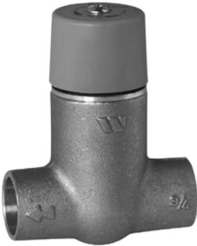
Honeywell FlowChecks prevent the flow of water to any part of a system when the pump is shut off. They permit summer/winter operation of indirect water heaters. Honeywell FlowChecks are easy to clean. Just unscrew the top of the valve for inspection and cleaning. Bronze and brass construction. To allow gravity flow, the FlowCheck can be changed to manual operation by turning the hand wheel counterclockwise (open position).
