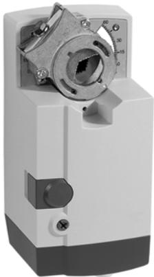
These direct-coupled damper actuators provide adjustable modulating control for: air dampers, air handling units, ventilation flaps, louvers, and reliable control for air damper applications with up to 4.6 m<sup>2</sup>/50 sq ft (seal-less dampers; air friction-dependent).
