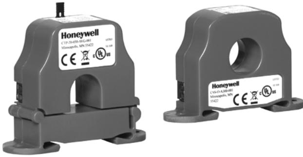
which can be monitored by a building management controller. These current sensors should be used in load trending (current monitoring) type applications. The split core transmitters are ideal for retrofit or existing installations, since it is not necessary to power down the unit and disconnect any wires during the installation process. Solid core transmitters are extremely easy to install, they are an excellent choice for new installations.
