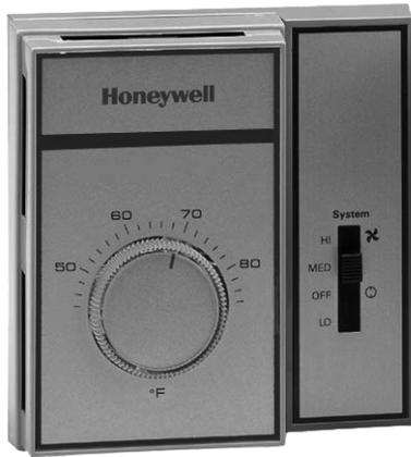
The T6169 thermostats control line voltage valves and/or blower motors on fan coil units in manual or automatic changeover, cooling, heating or cooling/heating systems. The thermostats feature a single fan and/or system manual switches.
