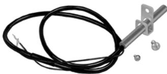
The T7022 Remote Temperature Sensor is a non-adjustable thermistor sensor. Its primary use is with the T7300 Programmable Commercial Thermostat (only in return air) to control heating or cooling equipment.
