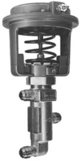
Three-pipe, sequencing, pneumatically operated water valve for controlling both hot and cold water flow in fan-coil and induction units. Replacement devices are available for Johnson, Powers, Robertshaw, Barber-Colman, and older Honeywell devices.
