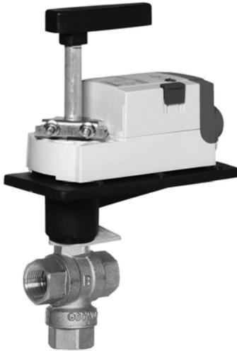
The VBN3 Three-Way Control Ball Valves control hot and chilled water with glycol solutions up to 50% in heating, ventilating, and air conditioning (HVAC) systems to provide two-position or modulating functions. These valve assemblies can be ordered with or without factory-mounted non-spring return or spring return direct-coupled actuators (DCA).
