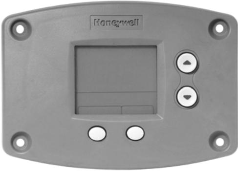
The S7910 Local Keyboard display interface provides setpoint and control adjustments to parameters of the R7910 SOLA Hydronic Control. All data is displayed on an LCD with backlight. The S7910 has four function buttons. The function of the bottom two buttons varies according to the operation mode and screen displayed. The right two buttons are used to adjust settings and navigate up and down the displayed data.
