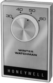
Used as a freeze warning device. Completes circuit to household lamp on temperature fall, indicating inoperative heating equipment.
