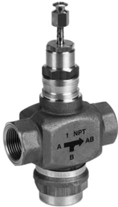
The V5013N is a three-way threaded globe valve that controls hot water, cold water, and glycol solutions (up to 50 percent concentration) in heating or cooling HVAC applications. The valves are used for mixing service to direct flow from one or two inlets to a common outlet in two-position or modulating control systems.
