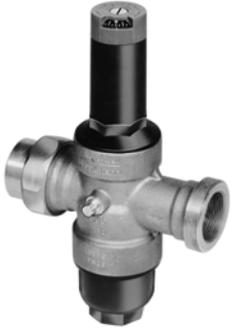
High quality pressure regulating valve that maintains a constant outlet pressure over a wide range of inlet supply pressures. Includes calibrated outlet pressure set dial that allows outlet pressure adjustments without the use of a gauge in most applications. Easy DialSet® Adjustment (no gauge required)
