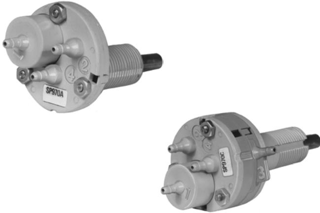
Used to manually position a remote damper actuator or to reset the setpoint of a pneumatic controller. They can also provide minimum damper position by setting a minimum pressure limit in the branch line to the damper actuator. Replacement kits are available for Johnson, Powers, Robertshaw, Barber-Colman, and older Honeywell switches.
