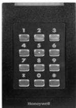
OmniClass™ OM56BHONA reader/keypad is built upon the convenience and reliability of prox technology and reads both 125 kHz Prox and 13.56 MHz Smart cards. Keypad is backlit for easy visibility in low-light conditions. LED bar at top of reader makes ADA compliant with built-in audible beeper.
