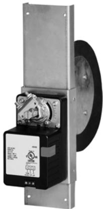
The RRD is a round damper that is easily inserted into rigid round ducts for retrofit zoning in forced air heating and cooling systems. It is available in four sizes for use in 5 in., 6 in., 7 in., and 8 in. ducts. The damper is used with Honeywell HZ221, HZ311, HZ322, HZ432 and similar zone control systems. The power open, power closed actuator draws 2 VA allowing multiple dampers per zone, but delivers high torque for reliable operation.
