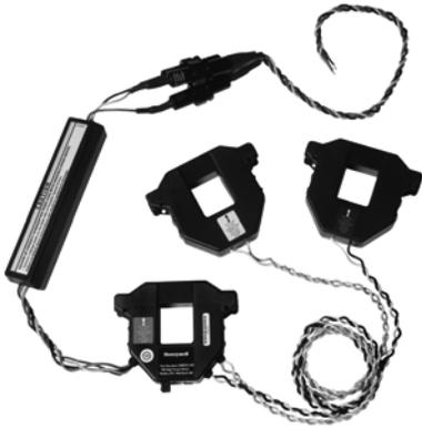
The Honeywell SXB40/SXB50 Series kW (real power)/kWh (consumption) transducers combine processing electronics and industrial grade CTs in an easy-to-install split-core package. These devices continuously measure voltage and current values for the monitored conductors and update calculations to provide highly accurate true RMS power readings. Models designed for balanced loads include one CT only, while models for unbalanced loads have three CTs.
