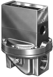
Solenoid-operated diaphragm valves provide slow opening and fast closing suitable for controlling natural, LP or manufactured gases. They are normally used on atmospheric boilers, commercial water heaters, and rooftop heaters.
