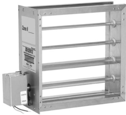
The ZD is a power close and spring open damper. It has a 24-volt motor used to control circulating air in heating, cooling and ventilating systems. It is used when a normally-open damper is required. The ZD is typically used with the TrueZONE systems and other electronic zoning systems.
