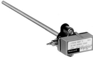
One-pipe, direct-acting temperature sensor used with RP908/ RP920 Controllers to provide proportional control of pneumatic valve or damper actuators. Rod and tube insertion element for duct, well, or through-the-wall mounting.
