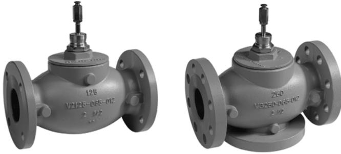
**VGf Flanged Globe Valves** are used for 2-position or modulating control of steam, hot water, or chilled water-glycol solutions up to 50 percent concentration in closed loop heating, ventilation and air conditioning (HVAC) systems. They can be operated by ML6984/7984, ML6420/6425, ML6421/7421 Electric Linear Actuators, MP953
