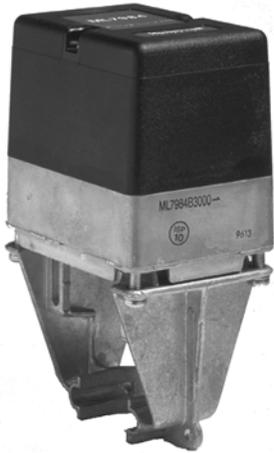
The ML7984 is a self-contained, self-adjusting, motorized linkage that mounts directly onto V5011 two-way or V5013 three-way valves and provides up to 25 mm (1") of linear stem travel. For use with Series 70 2-10Vdc, 4-20mA; Series 90 135 ohm; and Electronic (Super Mod) modulating signals controllers.
