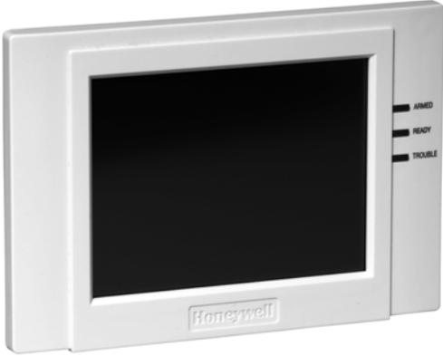
The S7999C is a four color touch-screen display module that provides an operator interface for monitoring and configuring parameters in the R7910 SOLA Hydronic or R7911 SOLA Steam system. The S7999C is flush mounted onto a panel by means of a mounting plate. Wiring connections to the S7999C are through a 4-pin wiring header.
