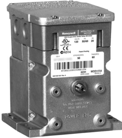
These Series 62 Modutrol IV™ Motors non-spring return floating control motors are used with controllers that provide a switched spdt or floating output to operate dampers or valves. These motors also have an internal electrically isolated feedback potentiometer that provides indication of the motor shaft position. Some models can be used for slaving Series 90 Motors.
