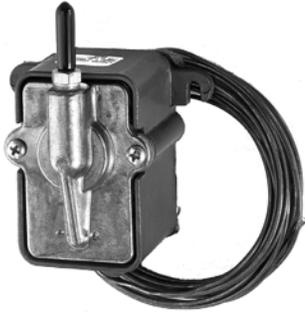
One-pipe, direct-acting temperature sensor used with RP908/ RP920 Controllers to provide proportional control of pneumatic valve or damper actuators. Averaging, liquid-filled element for duct mounting.
