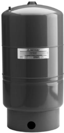
XPS Series (commercial) Expansion Tanks are designed to absorb hot water expansion in closed heating systems in larger installations. They are equipped with butyl diaphragms to separate clamped design. Pre-pressurized at 12 psi, the tank keeps fluids circulating and maintains minimum system pressure. Honeywell tanks resist waterlogging, loss of pressure through relief valves spills, loss BTUs for improved system performance.
