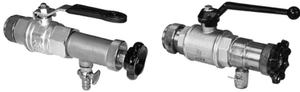
The MT110 Valve Cartridge Changing Tool enables the user to remove, and clean or replace the valve cartridge while the valve remains pressurized. Boiler shutdown is not required.
