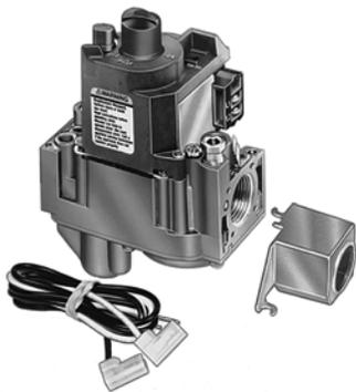
Combination gas control for use in 120 Vac, gas-fired, standing pilot appliances with capacities from 30 to 300 cfh.
