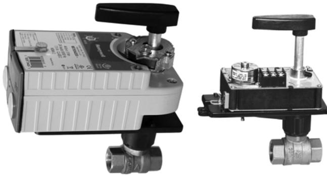
The VBN2 Two-Way Control Ball Valves control hot and chilled water with glycol solutions up to 50% in heating, ventilating, and air conditioning (HVAC) systems to provide two-position or modulating functions. These valve assemblies can be ordered with or without factory-mounted non-spring return or spring return direct-coupled actuators (DCA).
