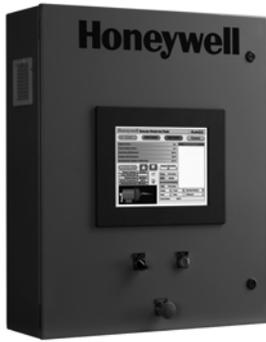
Delphi Combustion Efficiency Panel is a packaged, pre-wired panel with integrated color touchscreen display, flame safeguard control, linkageless fuel/air ratio control, oxygen trim and VFD capability. MF020-1-LC3 Oxygen sensor with mounting fitting and electrical connector and a Hall-effect sensor which monitors VFD driven blower and provides feedback to the control are included. System is set-up entirely via the touchscreen interface.
