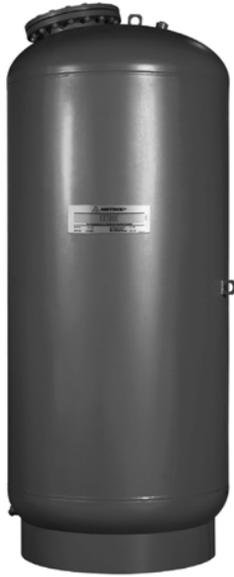
The Honeywell Thermal Expansion Absorber is a welded, pressurized expansion tank with a butyl diaphragm to control excess pressure in potable hot water systems. The Thermal Expansion Tank controls pressure build-up in the system, eliminates relief valve spillage, protects fixtures and extends water heater life.
