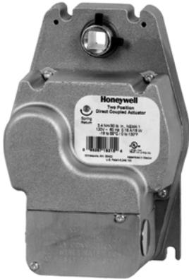
Spring return direct coupled actuators (DCA) for on/off damper control with an integral junction box. The actuator accepts an on/off signal from a single-pole, single-throw (SPST) controller. They are designed to operate reliably in smoke control systems requiring Underwriter's Laboratories Inc. UL555S ratings up to 350 F.
