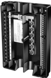
Provides terminals for field wiring for the R7999A ControLinks™ Fuel Air Controller. Terminals on the R7999A,B Controller engage the Q7999 contacts to make electrical connections. The Q7999A Subbase is panel-mounted.
