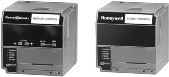
Microprocessor-based integrated burner control for automatically fired gas, oil, coal or combination fuel single burner applications. Provides safety, functional capability and features beyond conventional controls. With Valve Proving Feature. RM7800L comes standard with S7800A1142 Keyboard Display.
