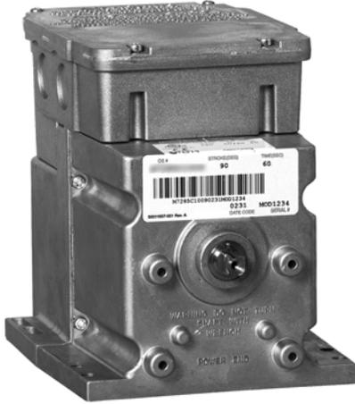
Series 62 Modutrol IV™ Motors are spring return floating control motors used with controllers that provide a switched spdt or floating output to operate dampers or valves. These motors also have an internal electrically isolated feedback potentiometer that provides indication of the motor shaft position and can be used for slaving Series 90 motors or rebalancing an external control circuit.
