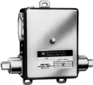
The P906 controllers respond to increases and decreases in pressure difference between high and low pressures in water or steam systems. The P906 provides proportional control in low voltage circuits and can be used to control a proportional valve to maintain desired pressure difference between two points in a system.
