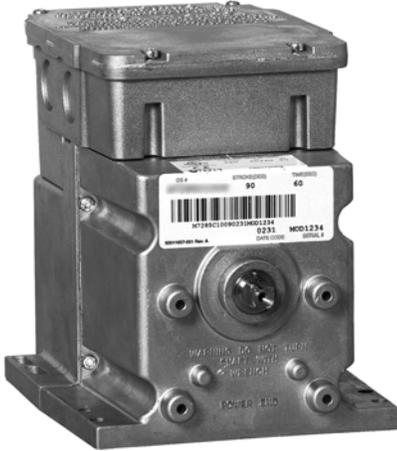
**Series 90 Modutrol™ Motors are spring return modulating proportional control motors used with controllers that provide a Series 90 output to operate dampers or valves.**
