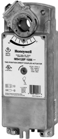
Spring return direct coupled actuators (DCA) for on/off damper control with an integral junction box. The actuator accepts an on/off signal from a single-pole, single-throw (SPST) controller. They are designed to operate reliably in smoke control systems requiring Underwriter's Laboratories Inc. UL555S ratings up to 350 F.
