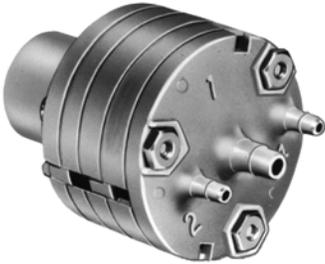
A modulating relay suitable for all types of heating and air conditioning control systems to reverse and increase the capacity of the branchline pressure to the final control element. The output varies inversely with the input with an adjustable offset. Replacement devices are available for Johnson, Powers, Robertshaw, Barber-Colman, and older Honeywell devices.
