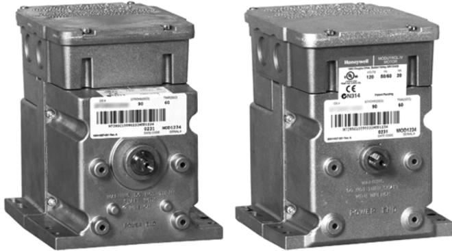
Series 72 Modutrol IV Motors are spring return and non-spring return motors (per motor type) used to control dampers and valves. The motors accept a current or voltage signal from an electronic controller to position a damper or valve at any point between open and closed.
