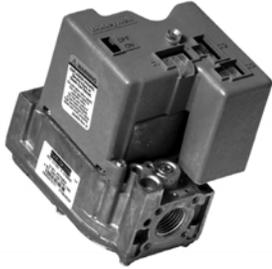
The SV9510 SmartValve System Controls combine gas flow control and electronic direct main burner ignition sequencing functions into a single unit. The ignition source is 120V hot surface igniter lighting the main burner flame. Provides all gas ignition safety functions by controlling gas flow, ignition source, and a 120 Vac
