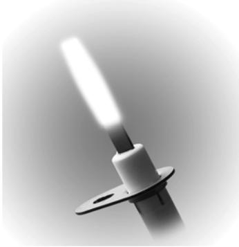
The Q3200U Universal Hot Surface Igniter Kit is designed to provide a robust field service replacement igniter in gas fired appliances with Norton/St Gobain 120 VAC silicon carbide hot surface igniters. The Q3200U uses a 120 volt silicon nitride igniter design with long life and high resistance to damage or burn out in the appliance.
