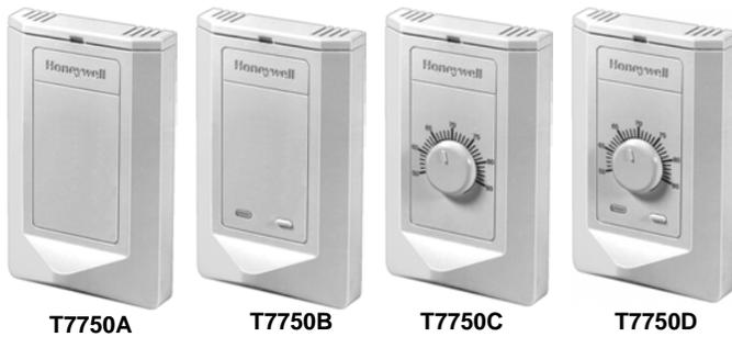
Temperature sensors for use with Excel 10 Series 1000 Controllers. The T7750 Wall Modules provide the following additional combination of options to the customer: analog setpoint input and for models used with Excel 10 Controllers, override (bypass) digital input contact, LED status indicator and network access jack.
