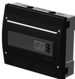
The AQ254 Add-a-Temperature Expansion Control Panel is used in conjunction with an AQ250, AQ25A, AQ251 or AQ252 Control Panel. It provides one additional loop temperature control capability for the AQ2000 control panel it is connected to and expands the total network capacity by up to 16 zones when used with AQ255 and/or AQ257 zoning panels.
