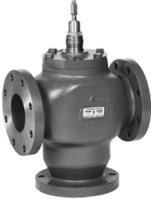
The V5013B are three-way mixing valves. The V5013C are three-way diverting valves. These valves provide proportional or two-position control of hot or chilled water in closed loop heating or cooling systems. These valves are offered in sizes 2 1/2 in. through 6 in.
