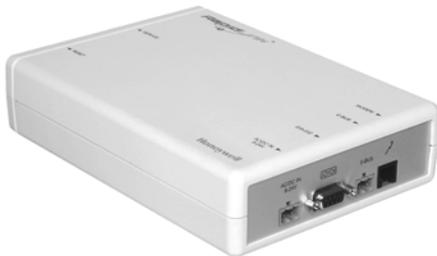
The Excel 10 Q7770A RapidLink device is a complete network interface unit for a FTT LonWorks® Bus network. RapidLink is equipped with an on-board modem that eliminates the requirement for an on-site modem for remote connections. The Q7770A uses 9 to 24 Vac or Vdc, 9 Vdc power supply using removable screw terminals or a 9 Vdc barrel connector to perform network operations. A connector cable attaches the Q7770A to the LonWorks-Bus port on Excel 10 controllers or wall modules.
