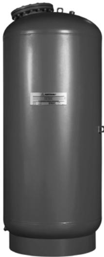
The Honeywell Thermal Expansion Absorber is a welded, pressurized expansion tank with a butyl diaphragm to control excess pressure in potable hot water systems. The Thermal Expansion Tanks controls pressure build-up in the system, eliminates relief valve spillage, protects fixtures and extends water heater life.
