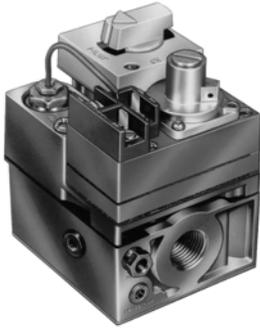
These gas controls combine a Lite-Rite manual gas cock, safety shutoff Pilotstat assembly, millivoltage automatic valve operator, and optional gas pressure regulator. They require the use of a 750 mv Powerpile generator (thermopile). The generator, heated by the pilot burner flame, provides the electrical energy to operate the combination gas control. A millivoltage thermostat with suitable accessory controls completes the automatic control system for the heating appliance.
