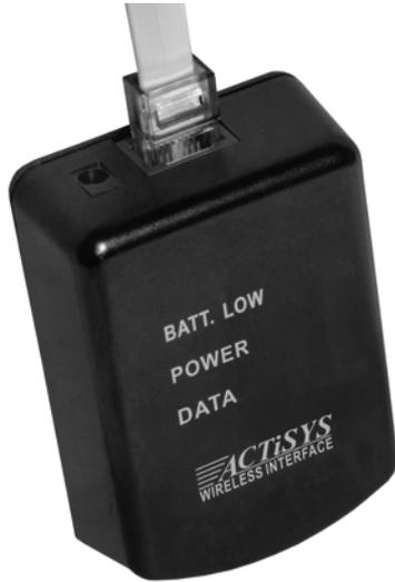
This InfraRed Thermostat Interface Module (IR-TIM) allows a PDA to be connected wirelessly to the T7350 Thermostat.
