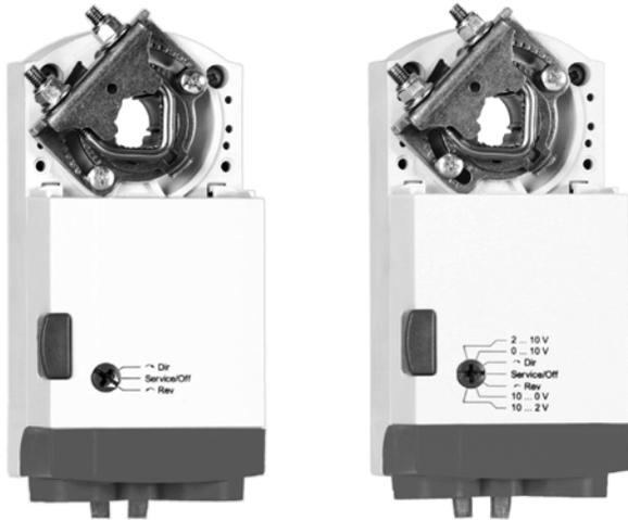
This non-spring return direct-coupled damper actuator provides modulating and floating/2-position control for: air dampers, air handlers, ventilation flaps, louvers, and reliable control for air damper applications with up to 10 sq. ft./ 44lb.-in. (5 Nm) and 20 sq. ft./88 lb.-in. (10 Nm) (seal-less damper blades; air friction-dependent).
