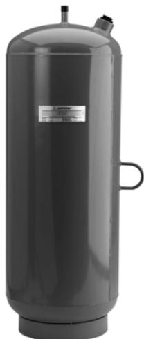
TAX Series (commercial) Expansion Tanks are designed to absorb hot water expansion in closed heating systems. TAX tanks are used in large installations. They are equipped with butyl diaphragms to separate the air from the system water (glycol). The tanks are a welded, not clamped, design. Pre-pressurized at 12 psi, the tank keeps fluids circulating and maintains minimum system pressure. Honeywell tanks resist waterlogging, loss of pressure through relief valve spills, and loss of BTUs.
