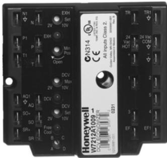
**W7212, W7213, and W7214 Economizer Logic Modules are used with C7232 Demand Control Ventilation (DCV) Sensors, and solid state C7400 Enthalpy Sensors or C7660 Dry Bulb Temperature Sensors. All models proportion outdoor and return air dampers for control of free cooling in commercial HVAC equipment.**
