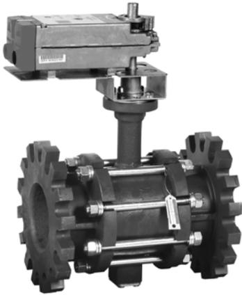
The VBF2 Two-Way Ball Valve Assemblies, with and without actuators, control hot and chilled water with glycol solutions up to 50% in closed loop heating, ventilating, and air conditioning (HVAC) systems to provide two-position or modulating functions. These valve assemblies can be ordered with or without factory-mounted non-spring return or spring return direct-coupled actuators (DCA).
