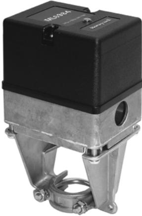
The ML6984 is a self-contained, self-adjusting, motorized linkage that mounts directly onto V5011 two-way or V5013 three-way valves and provides up to 25 mm (1") of linear travel (stem lift). For use with low voltage 3-wire SPDT Series 20 (on-off); Series 60 (floating) electromechanical (dry) contacts; or electronic (triac output) controllers (3-wire installation).
