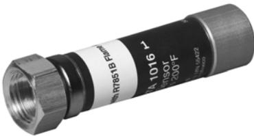
The Solid State Ultraviolet Flame Detectors detect the ultraviolet radiation emitted by combustion flames. The flame detectors are used with Honeywell flame safeguard controls to provide flame supervision for gas, oil, or combination gas-oil burners.
