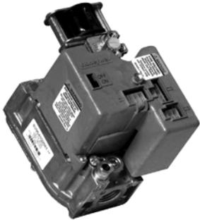
The TRADELINE® SV9541 SmartValve System Controls combine gas flow control and electronic intermittent pilot sequencing functions into a single unit. The Q3450 or Q3480 Pilot hardware supplies the low voltage igniter, flame sensor and pilot burner. These ignition system controls provide all gas ignition safety
