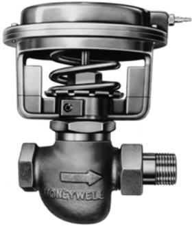
A normally open, single seated, straight-through or angle globe valve used for proportional control of steam or hot water in unit ventilator applications. Replacement devices are available for Johnson, Powers, Robertshaw, Barber-Colman, and older Honeywell devices.
