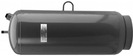
TAX Series (commercial) Expansion Tanks are designed to absorb hot water expansion in closed heating systems. TAX tanks are used in large installations. They are equipped with butyl diaphragms to separate the air from the system water (glycol). The tanks are a welded, not clamped, design. Pre-pressurized at 12 psi, the tank keeps fluids circulating and maintains minimum system pressure. Honeywell tanks resist waterlogging, loss of pressure through relief valve spills, and loss of BTUs.
