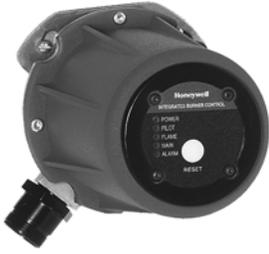
The CR7890B Integrated Burner Control consists of a self contained relay module, amplifier and a shutter type solid state Ultraviolet Detector for sensing the ultraviolet radiation generated by the combustion of gas, oil, or other fuels.
