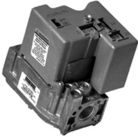
The SV9520 SmartValve System Controls combine gas flow control and electronic direct main burner ignition sequencing functions into a single unit. The ignition source is 120V hot surface igniter lighting the main burner flame. Provides all gas ignition safety functions by controlling gas flow, ignition source, and a 120 Vac
