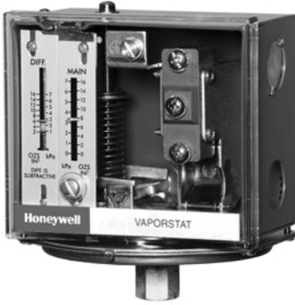
Provide operating control and automatic high limit protection for vapor heating systems with pressures up to 4 psi (8 kPa). All models have Microswitch snap switches to open or close a circuit on a pressure rise.
