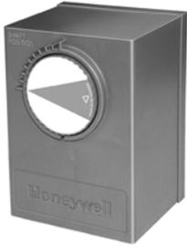
Provides 100 lb-in. torque, pulse-width-modulating (PWM) control of combustion air dampers, butterfly gas valves, oil modulation valves, and flue gas recirculation systems. The actuator includes a precision feedback potentiometer and integral power supply. The ML7999A Actuator is part of the ControLinks™ Fuel Air Control System, and must be used with the R7999 Fuel Air Controller.
