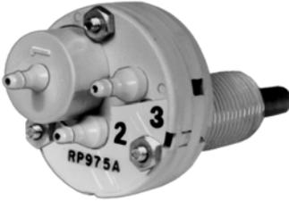
A three-port hesitation relay provides minimum outside air damper position plus controlled ventilation for large volume unit ventilators. Replacement devices are available for Johnson, Powers, and Barber-Colman devices.
