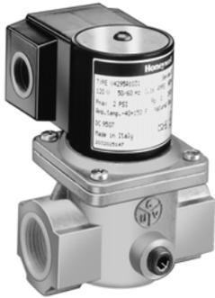
V4295A/V8295A are normally closed and V4295S/V8295S are normally open (vent) solenoid gas valve. Suitable for use on furnaces, ovens, atmospheric burners, commercial water heaters, roof-top make-up air units, power burners, and commercial/ industrial boilers.
