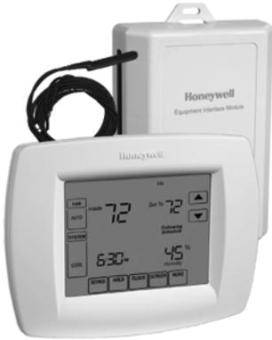
The VisionPRO IAQ touchscreen universal programmable thermostat provides electronic control of 24 Vac heating and cooling systems in addition to humidification, dehumidification and ventilation all with just 3 wires to the thermostat.
