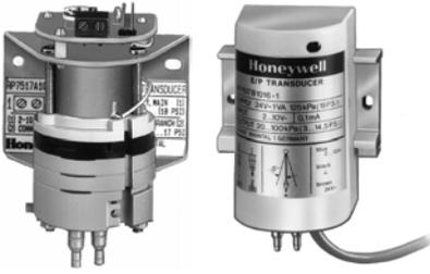
Electronic-Pneumatic Transducers are used in electronic-pneumatic control systems to convert a proportional electric output signal from a controller into a direct-acting, proportional pneumatic signal.
