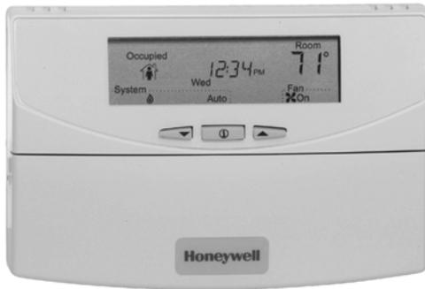
The T7351 Commercial Programmable Thermostat controls 24 Vac commercial single zone heating, ventilating and air conditioning (HVAC) equipment. The T7351 consists of a thermostat and subbase. The thermostat includes the keypad and display for 365-day programming. The subbase includes equipment control connections. The subbase mounts on the wall and the thermostat mounts to the subbase.
