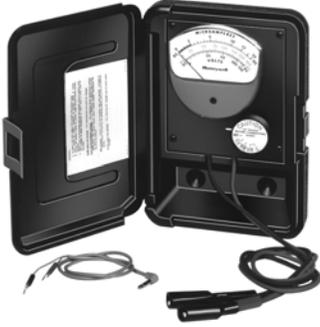
Combination ac/dc voltmeter and dc micrometer used to test all flame safeguard controls and associated burner equipment. The W136A can be used to verify flame detector output is sufficient to operate the flame relay.
