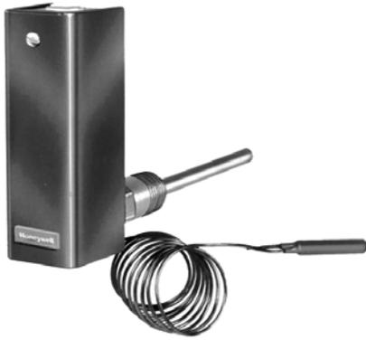
**L8100A,B, and C are immersion type controllers for regulating and limiting the tank temperature in water heaters. As the water temperature rises past the setpoint, the controller switches off the gas valve.**
