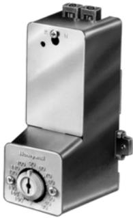
Two-pipe, single temperature, pneumatic temperature controller used to provide proportional control of pneumatic valves and damper actuators in heating and air conditioning systems. Replacement devices are available for Johnson, Powers, Robertshaw, Barber-Colman, and older Honeywell two-pipe pneumatic temperature controller.
