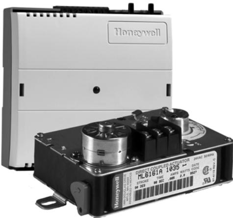
The W7751F2003 VAV II Controller is from the Excel 10 family product line. VAV controllers provide pressure independent or pressure dependent air flow control and series and parallel (induction) fan control using single and dual applications. The W7751F controllers provide additional outputs that control VAV box reheat coils. The ML6161B2024 is used to control dampers in VAV terminal units and for mounting on ball valves.
