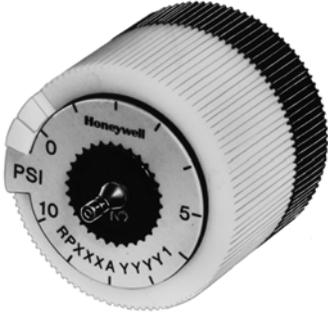
A four port non-bleed pneumatic relay which produces a modulating pressure output, proportional in a fixed ratio to pilot input changes. It is used to control pneumatic valve or damper actuators in sequence from a single thermostat. Replacement devices are available for Johnson, Powers, Robertshaw, Barber-Colman, and older Honeywell devices.
