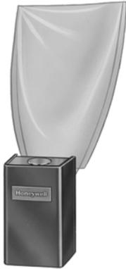
The Sail Switch activates an electronic air cleaner, a humidifier, or other equipment in response to airflow from the system fan. The S688A is mounted in the return air duct where the sail will be in the direct path of an unrestricted air stream.
