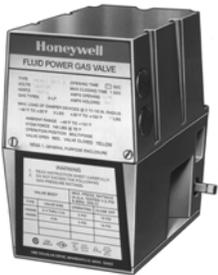
Use with V5055 or V5097 Gas Valves to control gas supply for commercial and industrial burners. Valve opens to low fire position when power is applied; valve opens all the way on demand.
