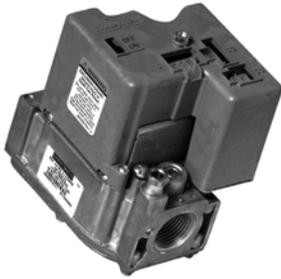
The TRADELINE® SV9641 SmartValve System Controls combine gas flow control and electronic intermittent pilot sequencing functions into a single unit. The Q3450 or Q3480 Pilot hardware supplies the low voltage igniter, flame sensor and pilot burner. These ignition system controls provide all gas ignition safety functions by controlling gas flow, ignition source, and a 120 Vac or
