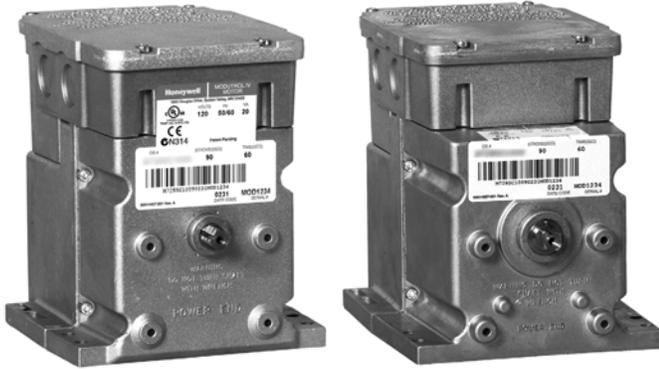
**Series 62 Modutrol IV™ Motors Spring Return and Non-Spring Return floating control motors used with controllers that provide a switched spdt or floating output to operate dampers or valves. These motors also have an internal electrically isolated feedback potentiometer that provides indication of the motor shaft position.**
