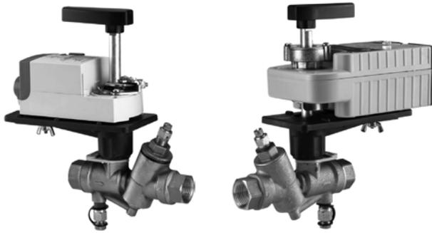
The VRN2 two-way dynamic pressure-regulating control ball valves maintain constant flow of hot or chilled water in closed loop heating, ventilating, and air conditioning (HVAC) systems regardless of head pressure fluctuations above the minimum specified pressure drop. These valve assemblies can be used with Honeywell non-spring return or spring return direct coupled actuators (DCA) with minimum torque of 35 lb-in (4 Nm) on valve sizes up to 3 inches (DN80).
