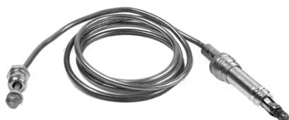
Thermocouples generate a thermoelectric current that senses a pilot flame on gas-fired heating systems. The pilot flame heats the tip of the thermocouple, producing a temperature differential between it and the base. This temperature difference generates a small amount of DC power, measured in millivolts.
