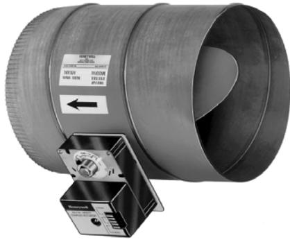
The DM7600 Commercial Zone Damper is used in zoning systems to control airflow in a round duct. A Honeywell ML6161 or ML7161 Direct Coupled Actuator is factory mounted to the damper to simplify field installation.
