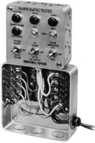
Provides quick operational check of Honeywell RA890 or R4795 nonprogramming primary controls.
