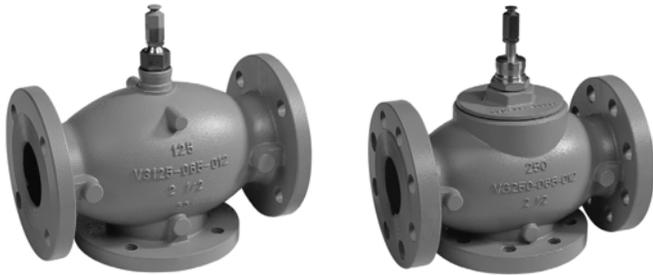
VGF Flanged Globe Valves are used for 2-position or modulating control of hot water or chilled water-glycol solutions up to 50% concentration in closed loop heating, ventilation and air conditioning (HVAC) systems. They can be operated by ML6984/7984, ML6420/6425, ML6421/7421 Electric Linear Actuators, MP953 Pneumatic Actuators, Modutrol™ Motors with Q5001 valve linkage, or MN/MS Series Direct Coupled Actuators with Q5020 or Q5022
