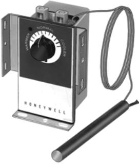
Two-pipe, single temperature, unit mounted, remote bulb pneumatic thermostat used to provide proportional control of pneumatic valves and damper actuators in heating and air conditioning systems.
