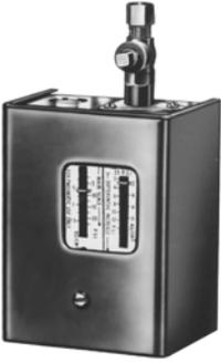
Used to convert a pneumatic signal from a controller to an electrical switching action to provide start and stop control of equipment such as fans and pumps. Replacement devices available for Johnson, Powers, Robertshaw, Barber-Colman, and older Honeywell pneumatic/electric switches. Adjustable setpoint.
