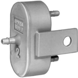
A three-port relay used in HVAC systems averages the signals from two thermostats to control a single device such as a heating coil valve for a multizone unit. The pneumatic averaging relay provides an output pressure equal to the average of two input pressures. Replacement devices are available for Johnson, Powers, Robertshaw, Barber-Colman, and older Honeywell devices.
