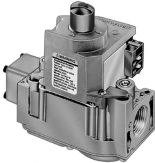
Combination gas control for use with hot surface/direct spark systems in 24 Vac, gas-fired appliances, with capacities from 30 to 415 cfh.
