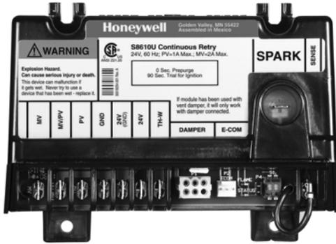
Field service replacement for most Honeywell, Robertshaw, Johnson, and UTEC (HSC) Intermittent Pilot Ignition Modules. Provides electronic control of most intermittent pilot ignition systems used on gas-fired furnaces, boilers, and other heating appliances.
