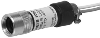
The C7962B Visible Light Flame Detector detects the visible light emitted by fuel oil combustion flames. The C7962B Detector is used with Honeywell Flame Safeguard controls to provide fuel oil flame supervision in commercial and industrial burners.
