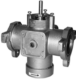
The V5197A is a firing rate valve used to provide variable flow control of air, natural gas, liquefied petroleum (LP), and manufactured gases. The V5197A is actuated by a ML7999A or B firing rate motor that can be mounted directly on the valve. The V5197A is not applicable as a safety shutoff valve. The V5197A is specially designed to provide fine control of gas flow in applications where a high turn down ratio is required. The maximum flow adjustment screw on the bottom of the valve allows
