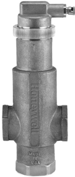
Conventional automatic air vents installed in Hydronic heating systems can leak and cause inefficient system operation. To effectively eliminate air from the system without bleeding, air bubbles need to be vented. The NEW Honeywell SuperVent purges air through a no clog vent assembly that controls dirt and debris to minimize air vent fouling.
