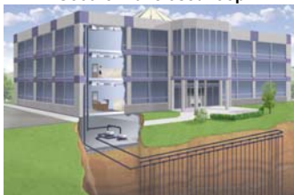
Geothermal closed loop
